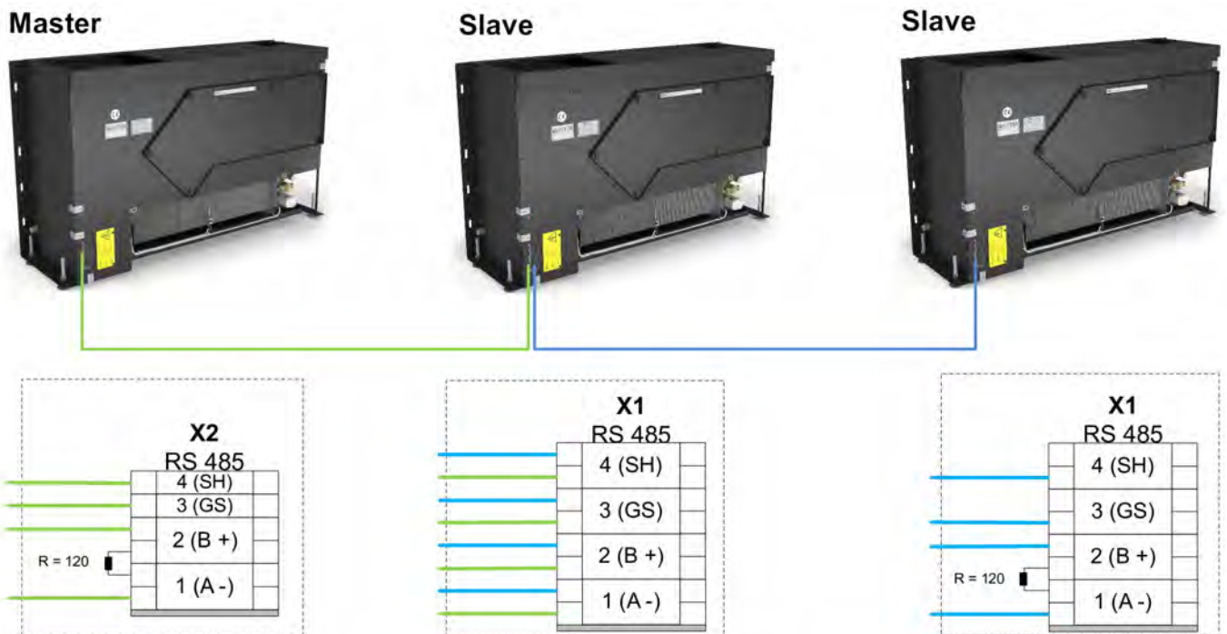
Fig. 22: FSL CONTROL III communication 3 devices
