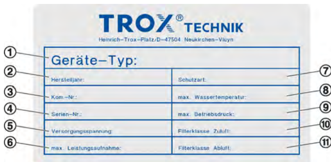
Fig. 39: The rating plate is affixed to the cover plate.
