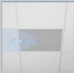
Horizontal one-way air discharge
