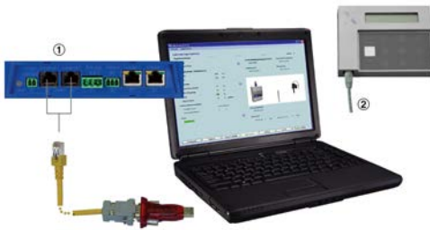
Fig. 9: PC connection via various interfaces
