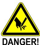
**The fans are delivered with inlet guards. If there is a danger of contact with the impeller owing to the way the fan is installed, then it is necessary to fit guards conforming to EN ISO 13857.**
