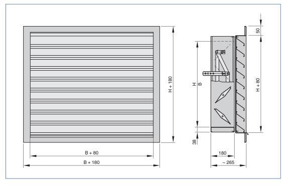
Illustration shows a multileaf damper with drive arm, operating side on the right
