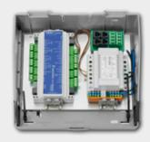
X-AIR-PCASE230V With additional components (by others) zone module / splitter
