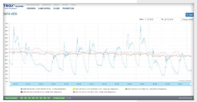
X-TAIRMINAL allows users to display and analyse all parameters for a ventilation and air conditioning system, for example to recognise trends.
