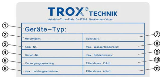
Fig. 33: The rating plate is affixed to the cover plate.
